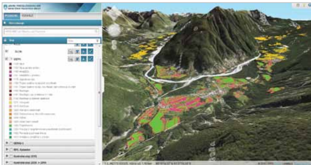
3D viewer combines aerial photography with a Digital Elevation Model or Digital Terrain and is augmented with various data layers, such as land use information.
